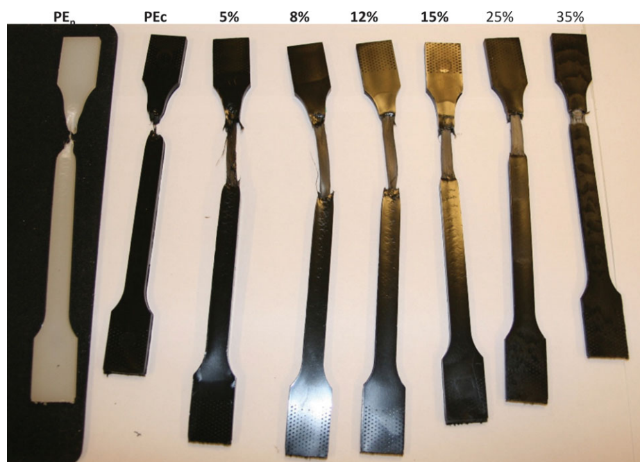
Figure 4. Individual test specimens after the tensile test. [Color figure can be viewed in the online issue, which is available at wileyonlinelibrary.com .]
